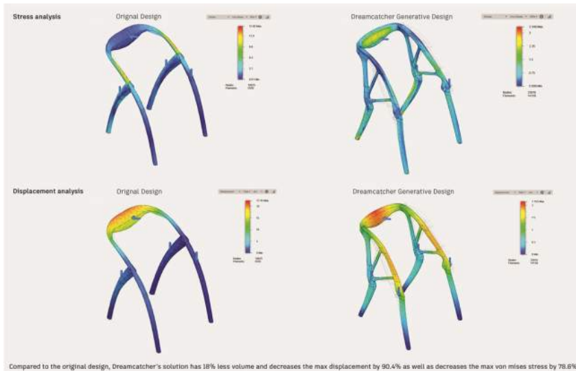
Compared to the original design, Dreamcatcher's solution has 18% less volume and decreases the max displacement by 90.4% as well as decreases the max von mises stress by 78.6%.
